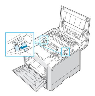
**6** Using the handle, lift the transfer belt out of the printer by lightly pulling it towards the left of the printer. Set it on a clean flat surface.
